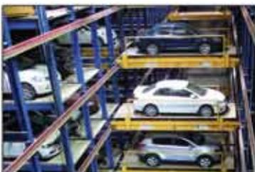
5. Robotic Parking Systems does the rest. The car is picked up by the computerized machinery and lifts that safely place it inside the building on a shelving system. The Ibn Battuta Gate facility handles 250 cars per hour with up to 32 cars in motion at any time.
